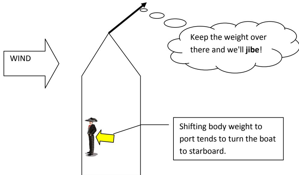
Similarly, shifting your weight to starboard will tend to make the boat turn toward port. Exploit this fact to do a turn in the opposite direction.
