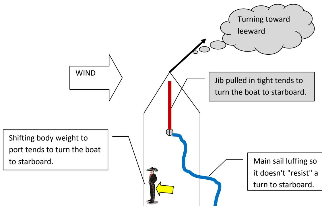
Just to sail straight, you will need to make continual minor adjustments in weight and sail trim. Sailing straight requires finding and maintaining an equilibrium where the boat has neutral helm. Due to the changing influences of the environment (i.e. wind, current, waves, etc.) you need to constantly adjust your weight and sail trim just to sail straight. This is what makes sailing rudderless challenging and skillful.
