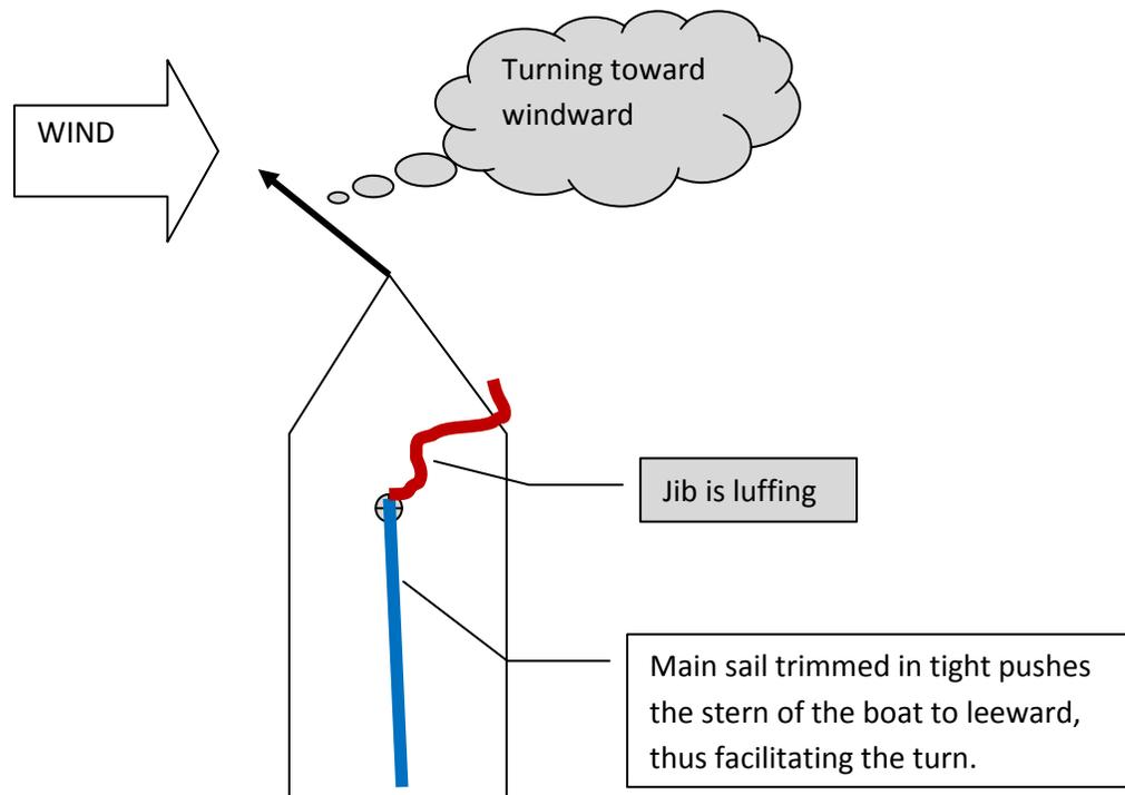
To complete a full turn to windward (ie. a tack), we simply maintain this sail trim until the bow of the boat is beyond the "point of no return" through the wind. Once the bow is beyond the point of no return, pull the jib in tight which will force the nose of the boat further downwind. This completes the turn.
