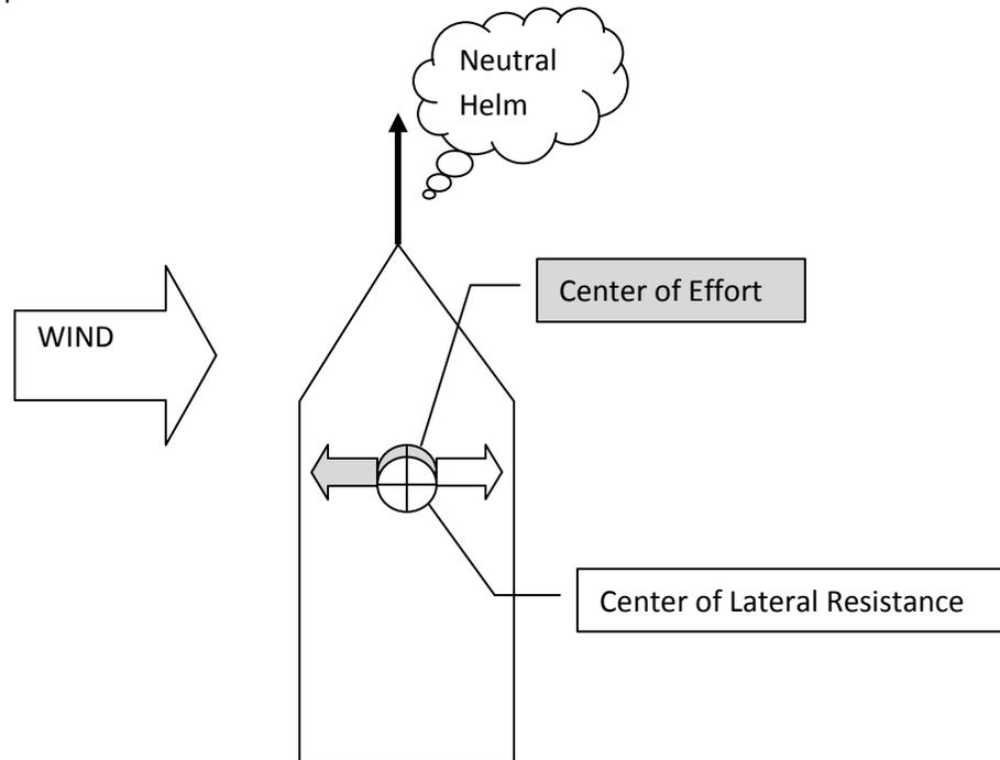
When sailing rudderless in a straight line, we try to keep the COE on top of the CLR.
